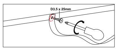
STEP 2: Make a hole on the wall and pull the wall plug in
