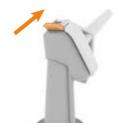
To remove the tool from the  $360^{\circ}$  connector, push the release tab at the front of the tool.
