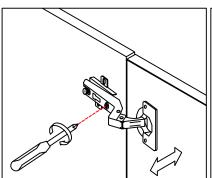
**A.**Lateral adjustment by screw adjusting
