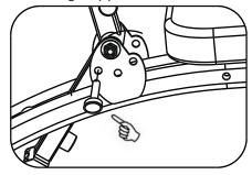
Unfold the seat back and fix it with the long pin.
