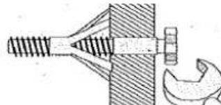
For use when fitting or supporting heavy loads such as shelving, wall cabinets, coat racks.
