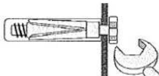
For use with heavier loads such as TV & HiFi Speakers and Satelite Dishes etc.
