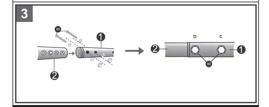
WARNING! Tube 2 must be fitted to tube 1 so that both M6 Bolts are secured tightly in the two available places. The Seesaw can be fitted in any of the three combinations: AB or BC or CD.
